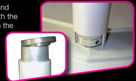
Only when the pole is true and vertical, can you wind up the jack to take the load. For round poles, wind up the capstan using a screwdriver (or similar) the holes provided. The preparation in the PVC-U sleeving described earlier allows access. For square poles, you obviously need to use a spanner or adjust the nut by hand.
